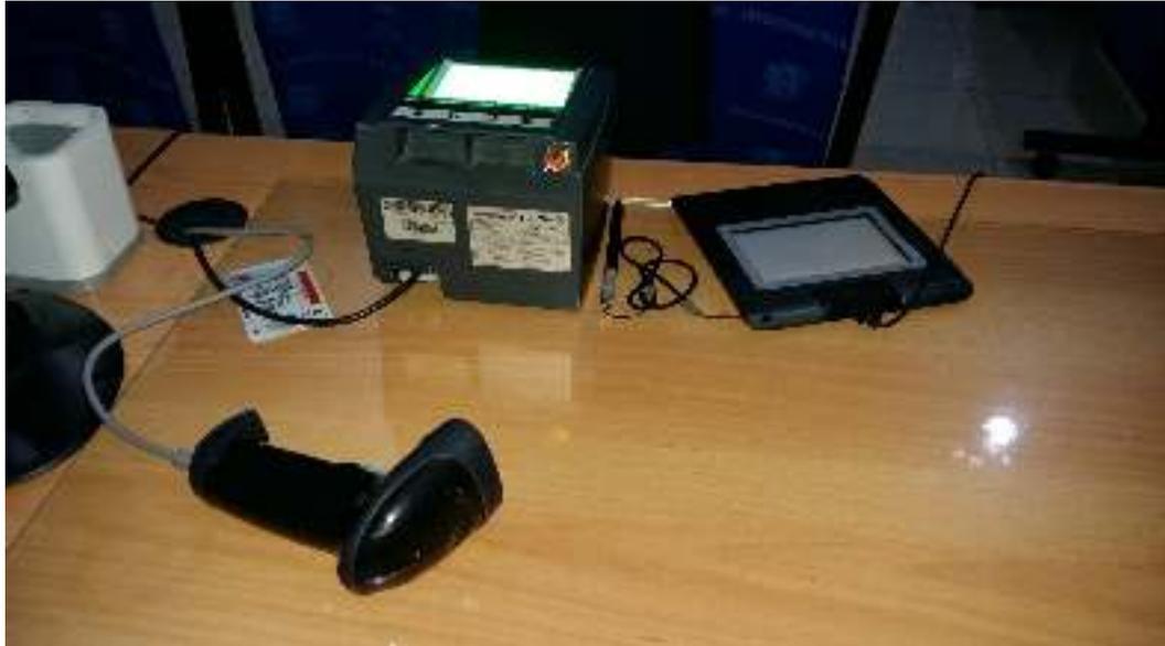
Gambar 11. *Barcode Scanner, Fingerprint Scanner, dan Signature Pad*
