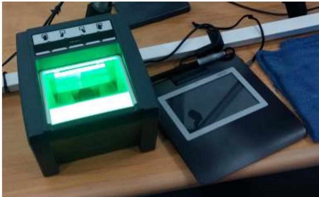
Gambar 31. Slap *Fingerprint Scanner* Crossmatch Patrol dan *Signature Pad* Wacom
