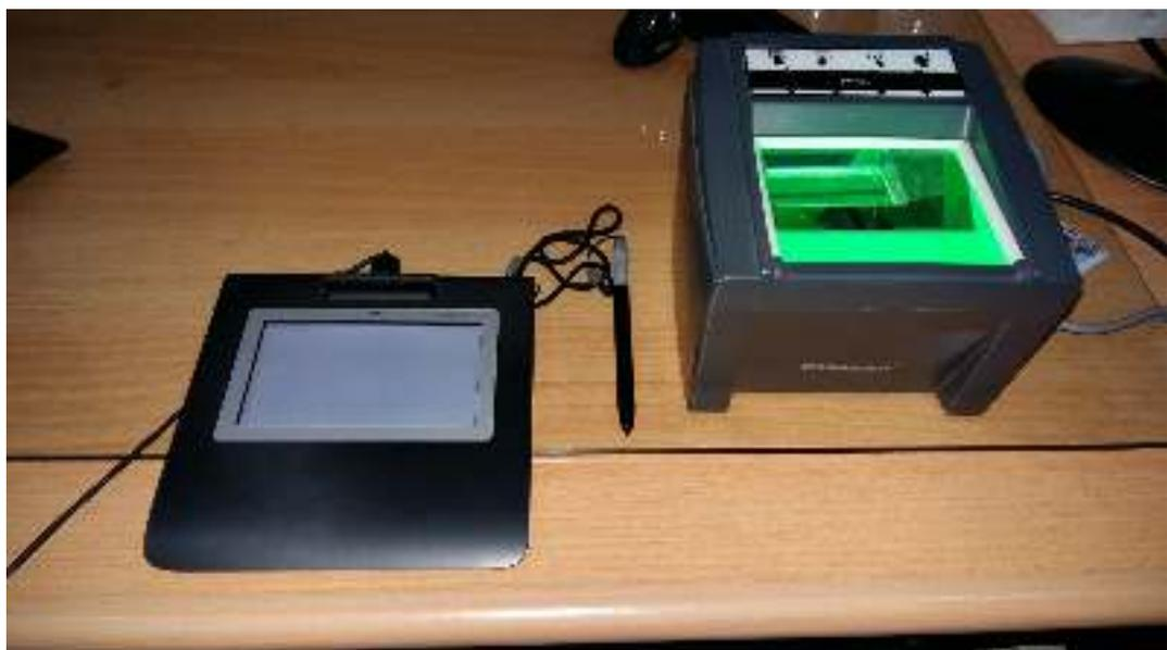
Gambar 10. *Signature Pad Wacom* dan Slap *Fingerprint Scanner* Crossmatch Patrol
